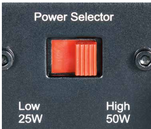
The Power Selector can be used to adjust tubes such as a 6550.
